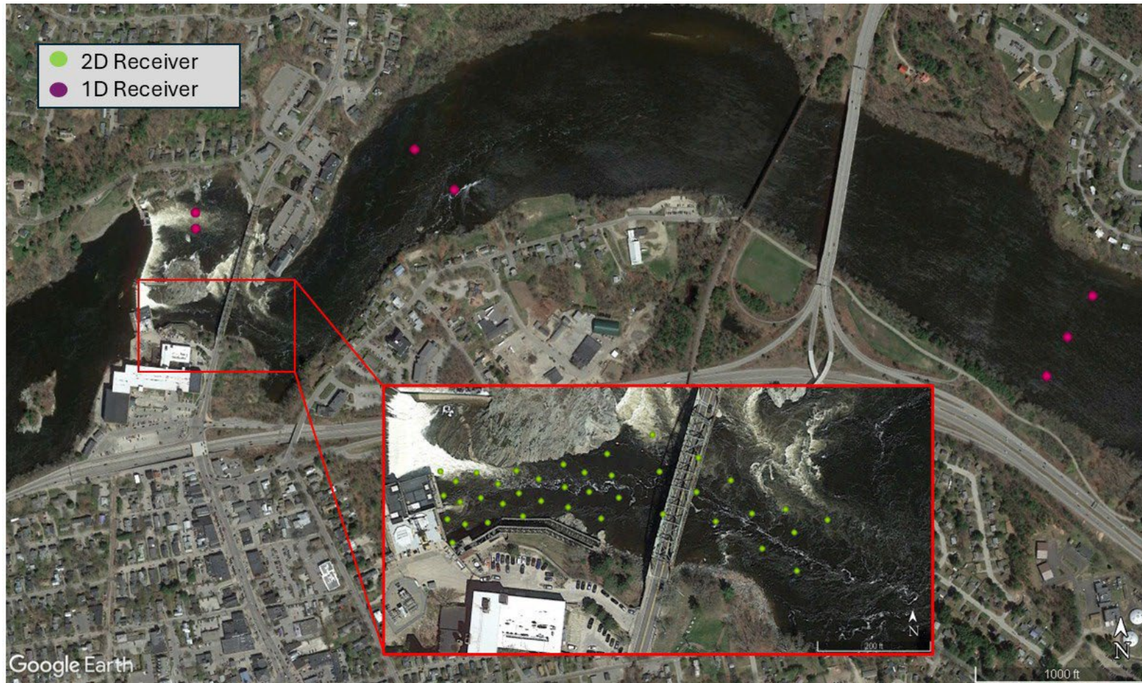
Figure A-1. Full Theoretical Acoustic Receiver Installation for Phase II of the Project Interaction Study at Brunswick
