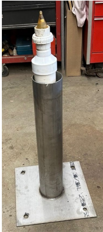
Figure A-3. Bottom Mount/Housing for ATS SR3001 JSATS Receivers to be Diver Installed During Phase II of the Project Interaction Study at Brunswick
