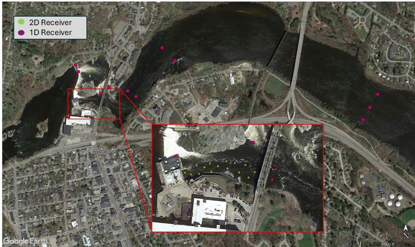
Figure A-2. Proposed Acoustic Receiver Installation for Phase II of the Project Interaction Study at Brunswick
